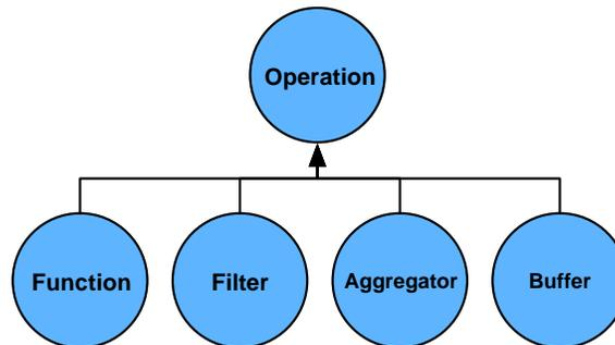
All Operations operate on an input argument `Tuple` and all Operations other than `Filter` may return zero or more `Tuple` object results. That is, a `Function` can parse a string and return a new `Tuple` for every value parsed out (one `Tuple` for each 'word'), or it may create a single `Tuple` with every parsed value as an element in the `Tuple` object (one `Tuple` with "first-name" and "last-name" fields).
