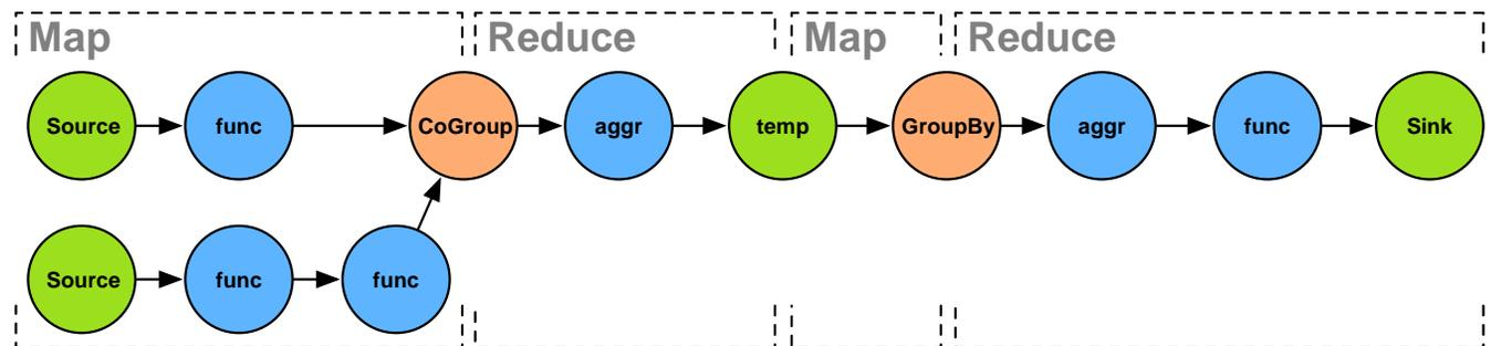
Above we can see how a reasonably normal Flow would be partitioned into MapReduce jobs. Every job is delimited by a temporary file that is the sink from the first job, and then the source to the next job.
