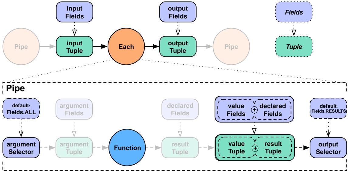
If the argument selector is not given, the whole input Tuple (`Fields.ALL`) is passed to the Operation as argument values. If the result selector is not given on an `Each` pipe, the Operation results are returned by default (`Fields.RESULTS`), replacing the input Tuple values in the tuple stream. This really only applies to `Functions`, as `Filters` either discard the input Tuple, or return the input Tuple intact. There is no opportunity to provide an output selector.
