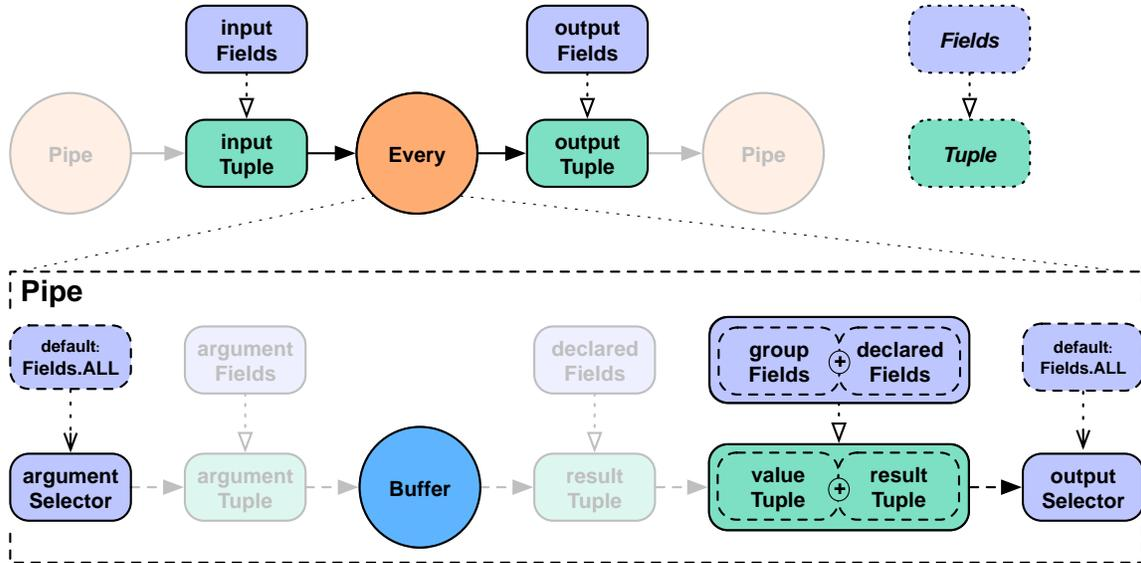
For the `Every` pipe when used with a `Buffer` the behavior is slightly different. Instead of associating the `Buffer` results with the current grouping `Tuple`, they are associated with the current values `Tuple`, just like an `Each` pipe does with a `Function`. This might be slightly more confusing, but provides much more flexibility.
