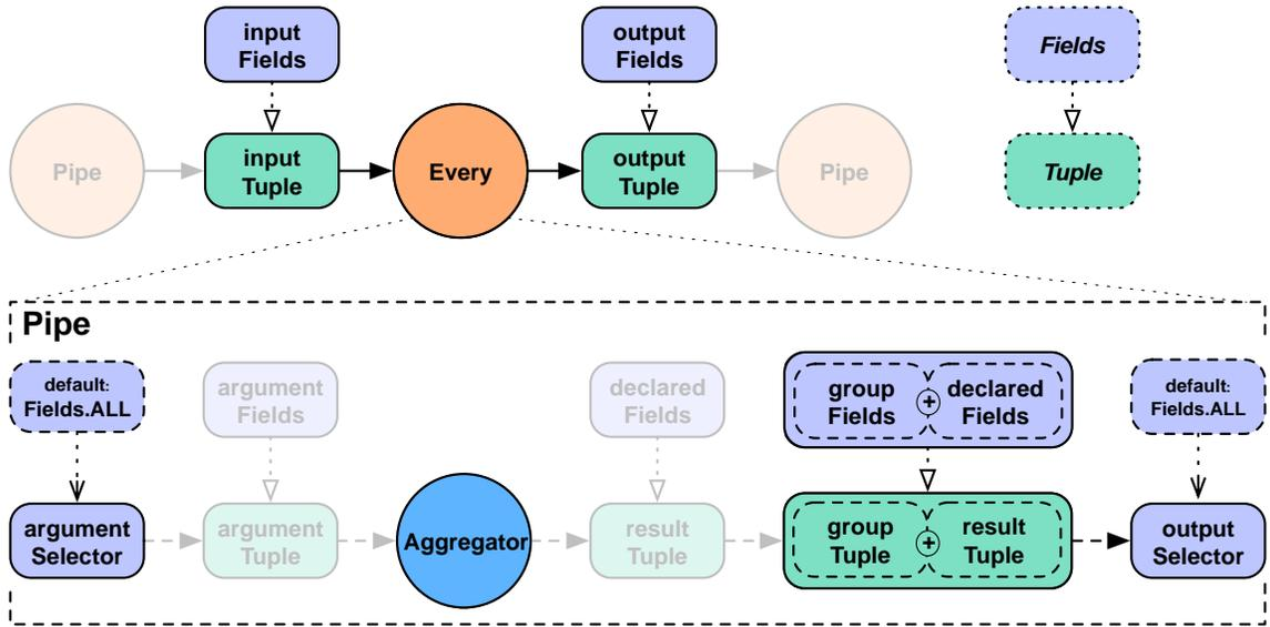
For the `Every` pipe, the `Aggregator` results are appended to the input Tuple (`Fields.ALL`) by default.
