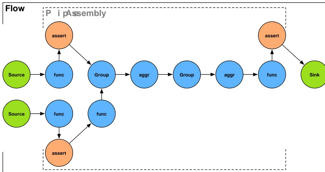
Stream assertions are simply a mechanism to 'assert' that one or more values in a tuple stream meet certain criteria. This is similar to the Java language 'assert' keyword, or a unit test. An example would be 'assert not null' or 'assert matches'.
