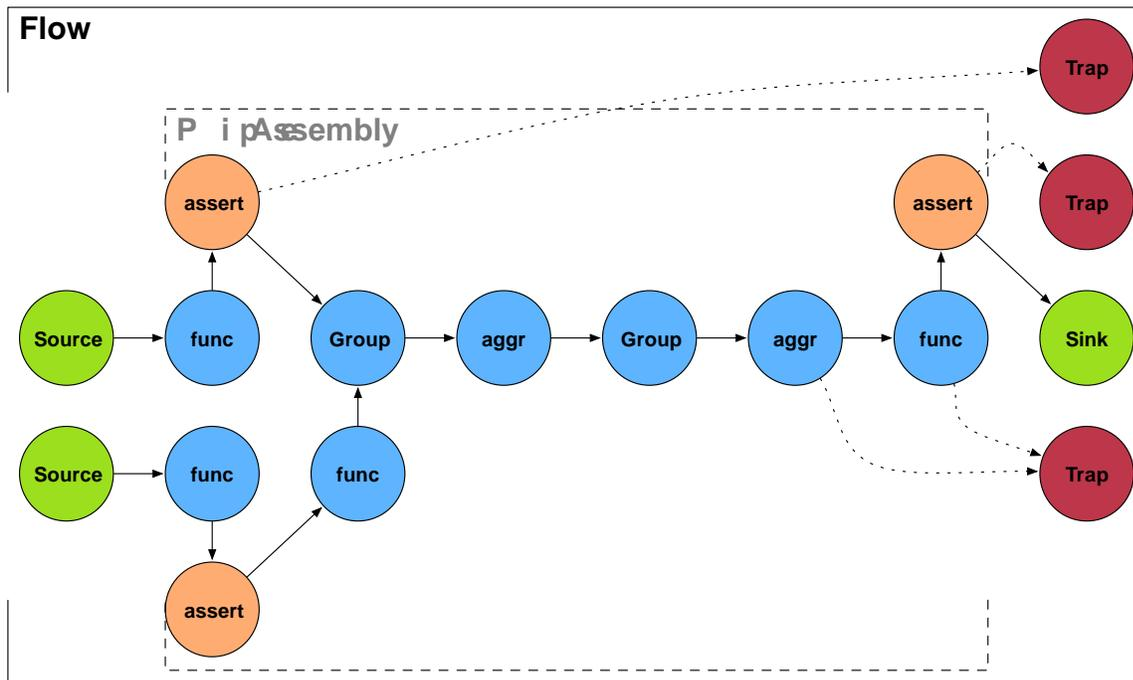
Failure Traps are the same as a Tap sink (opposed to a source), except being bound to a particular tail element of the pipe assembly, traps can be bound to intermediate pipe assembly segments, like to a Stream Assertion.
