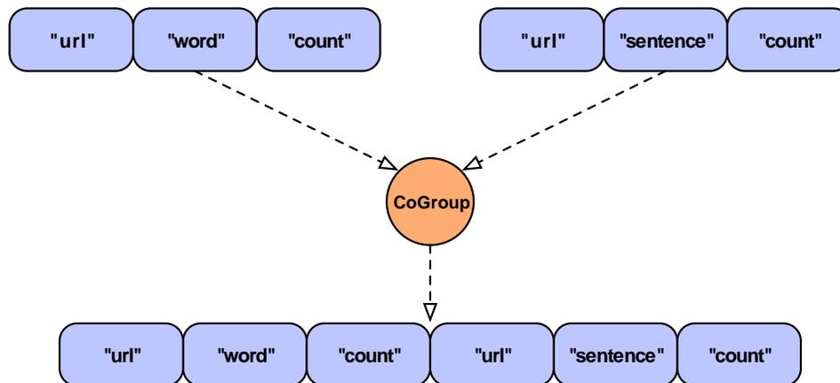
In the above example, we see what "logically" happens during a join. Here we join two streams on the "url" field which happens to be common to both streams. The result is simply two Tuple instances with the same "url" appended together into a new Tuple. In practice this would fail since the result Tuple has duplicate field names. The CoGroup pipe has the *declaredFields* argument allowing the developer to declare new unique field names for the resulting tuple.
