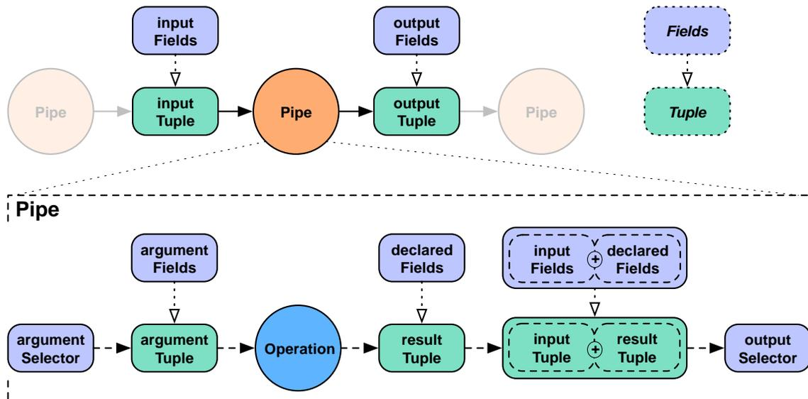
The "argument selector" selects values from the input `Tuple` to be passed to the `Operation` as argument values. Most `Operations` declare result fields, "declared fields" in the diagram. The "output selector" selects the output `Tuple` from an "appended" version of the input `Tuple` and the `Operation` result `Tuple`. This new output `Tuple` becomes the input `Tuple` to the next pipe in the pipe assembly.
